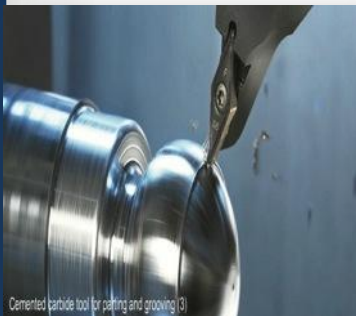
Cemented carbide tool for turning and grooving (3)
