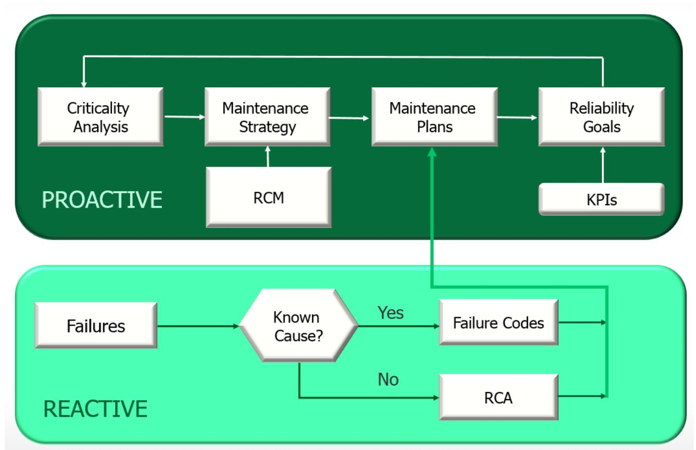
To better understand, let's look at the flow diagram above. Starting from the bottom, the part named "reactive", the first step is to understand why the equipment is failing. If we know the causes of failures, then we need to group them to identify what are the most important.
