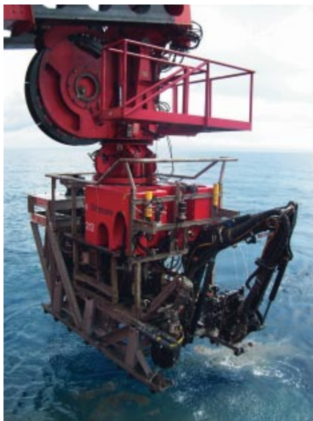
ROV fitted with rock cutter for bulk
