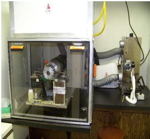
HFRR Lubricity Test Apparatus
