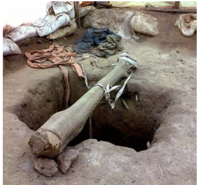
Miners use a rope attached to a beam stretched over the mouth of the pit as support to climb down into the pit or climb out. © Amnesty International and Afrewatch
