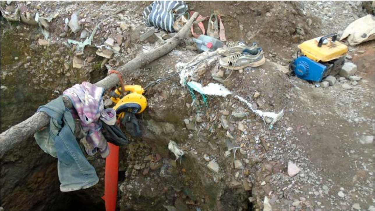
An air pump supplies oxygen to artisanal miners working in the pits in a mine on the outskirts of Kolwezi, DRC. A miner told researchers that when the generators run out of fuel, they cannot breathe and need to climb out as fast as possible, May 2015. © Amnesty International and Afrewatch
